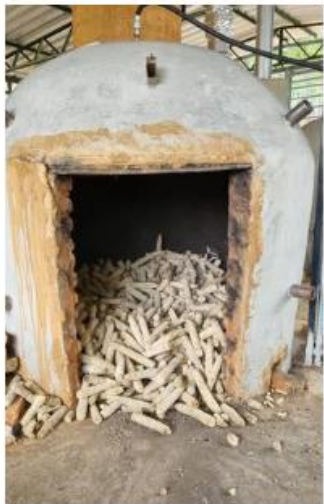
Filling the kilns with corn cobs
